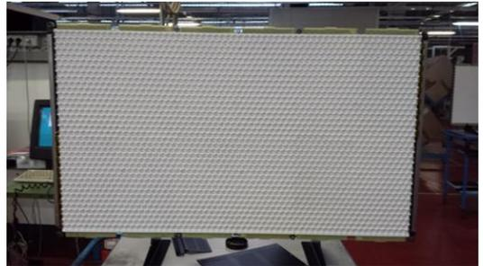
More in detail, a new reflector structure ("flowers") is under development. It has been simulated using optical CAD.
